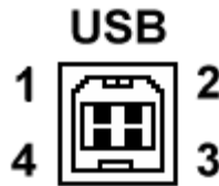
Figure 3-11: USB Connector Pin Orientation.
