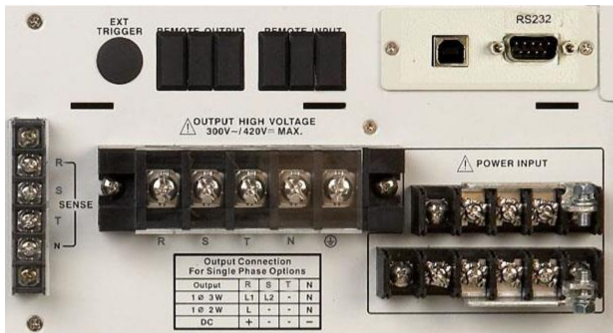
Figure 1: Input/Output Terminal Block and Output Connection Description
