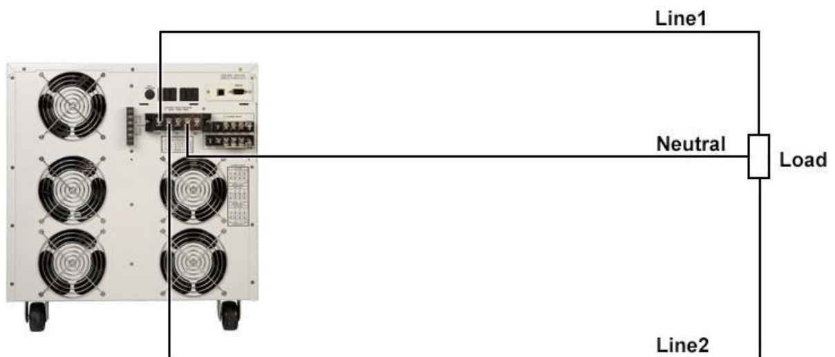
Figure 5: 1Ø3W Configuration
