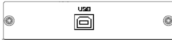
Fig 2-5 33611F Series USB Connection Rear panel
