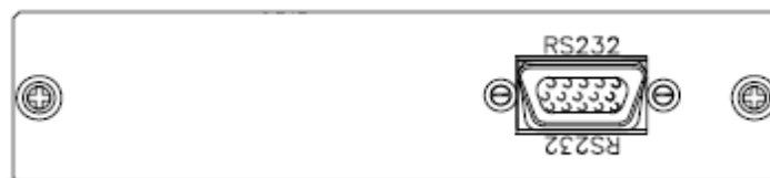
Fig 2-4 3305F RS232 Connection
