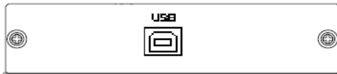
Fig 2-6 3302F USB Connection
