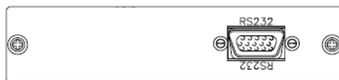
Fig 2-4 3302F RS232 Connection
