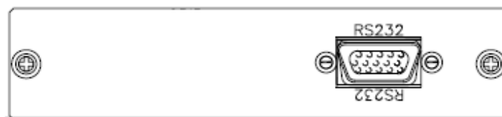
Fig 2-5 1000A RS232 Connection
